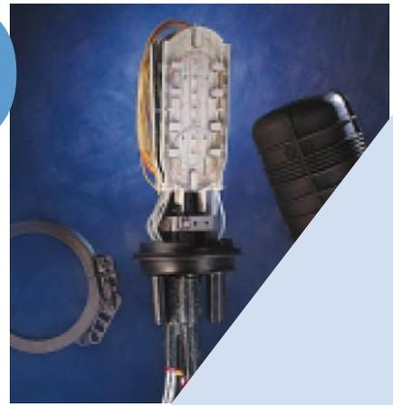
FOSC 400 closures combine proven fiber management hardware from the earlier FOSC 100 closures, with a completely new sealing system. Base-to-dome seals on FOSC 400 are mechanical for ease of installation and re-entry. Cable seals feature a new heat-shrink sleeve and hot melt adhesive system that is installed with a hot-air gun. Common materials, accessories and practices are used throughout the product line to simplify training, reduce inventory and enhance productivity.
